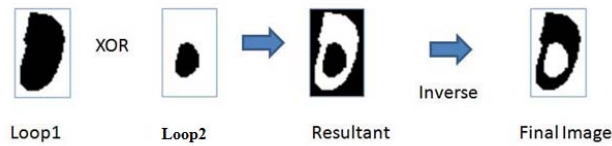
FIGURE 12. BOUNDARY FILLING OF MULTIPLE LOOPS
